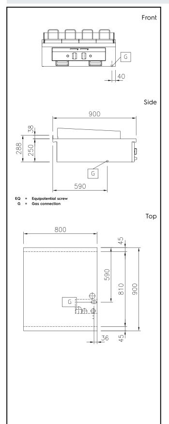
Gas Gas Power: 19 kW Gas Inlet: 1/2" **Key Information:** External dimensions, Width: 800 mm
